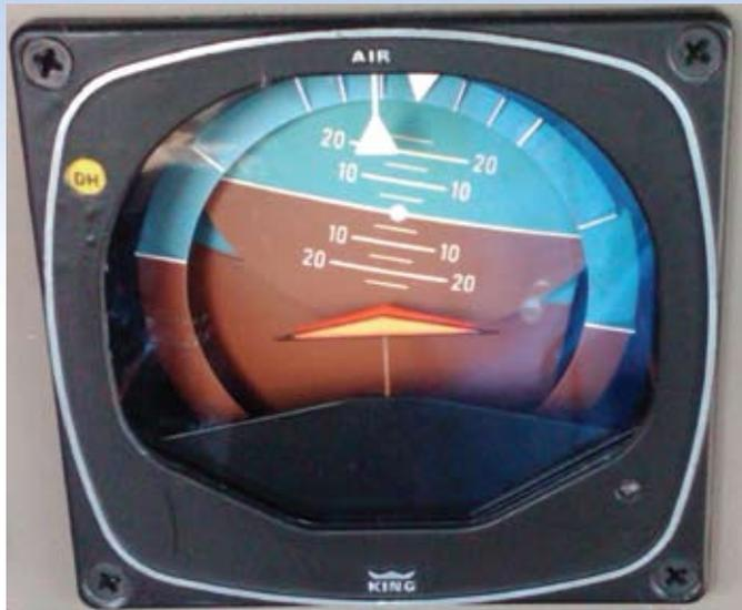
The solid state ADHRS is vastly more reliable than a mechanical attitude gyro and features internal failure detection that will disconnect the autopilot immediately
