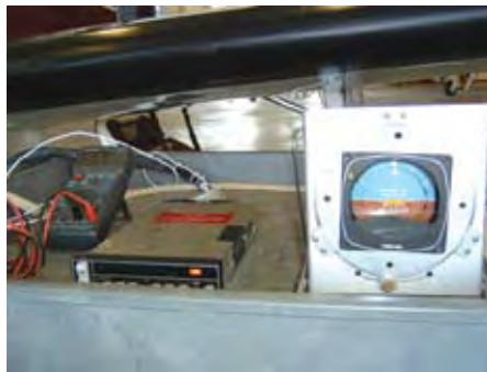
KI256 under autopilot calibration on bench
