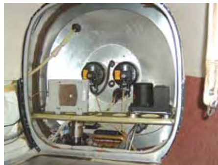
Outflow valves in avionics bay
