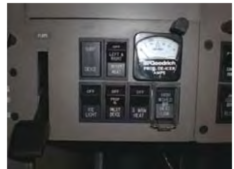
De-ice control switches
